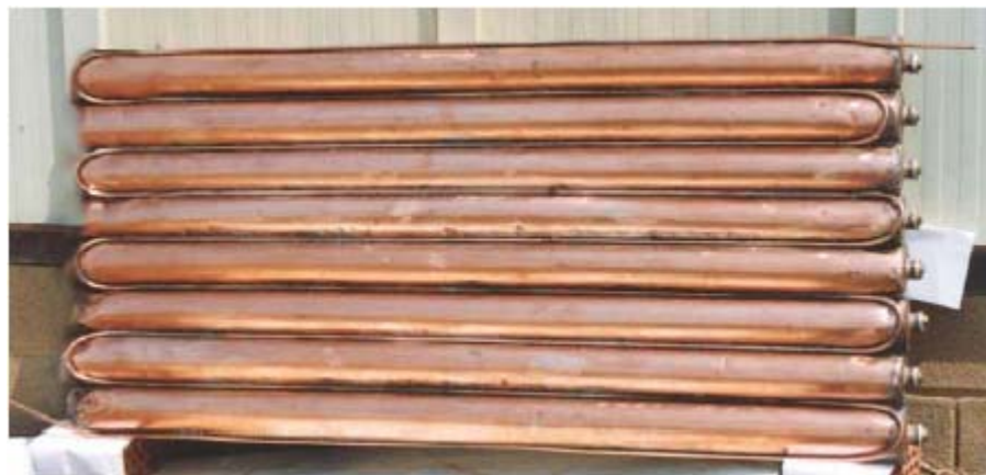
Fig. 17. The storage tank and the serpentine before treated to get the selective coating.
