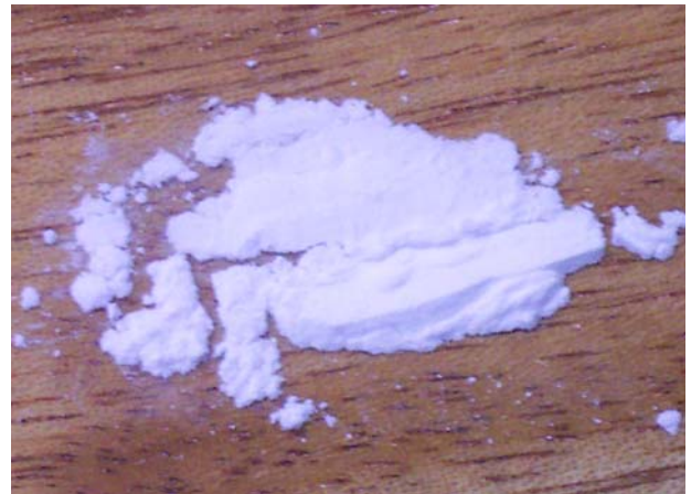
Fig. 27. Microencapsulated PCM commercialized by BASF.
