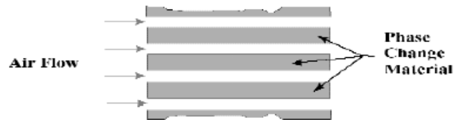
Fig. 8. Thermal storage unit with PCM.
