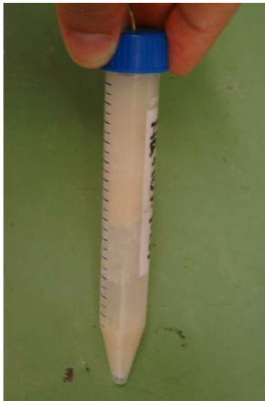
Fig. 24. Segregation of a salt hydrate.
