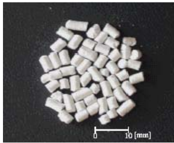
Fig. 9. Granulated PCM used by Takeda et al. [27].
