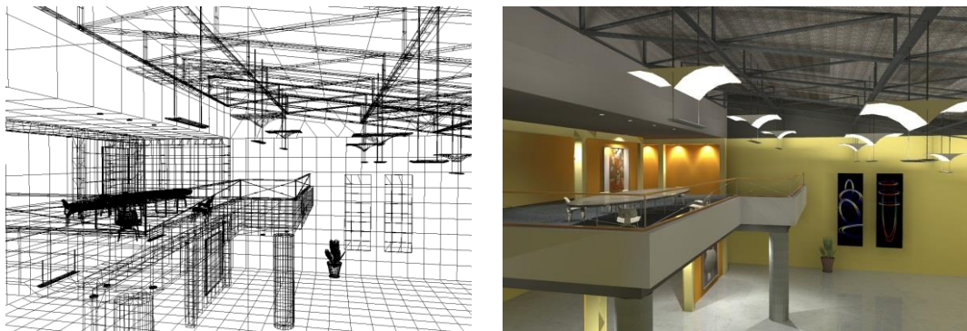
Figure 68: Model created in AGi32 – wireframe (left), Rendered: radiosity plus raytrace (right).
