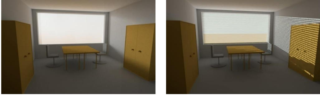
Figure 108: Simulation of a daylighting system represented by its BSDF (left) and by a combination of BSDF and geometry (right)
