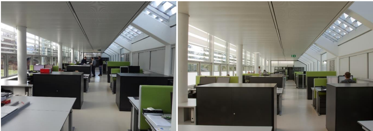
Figure 8: Interior view of example office at overcast conditions with movable systems retracted (left) and at sunny conditions with movable systems in positions to avoid direct sun penetration (right).
