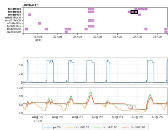
FIGURE 11. The graph shows measurement data related to the anomaly highlighted in the Anomaly heat map. Raised by a SunSearcher algorithm, the anomaly is likely caused by a rainy day resulting in unusually low-temperature readings (see lower plot) on the 24th of August. However, as this is typical behavior to the domain experts, it was not clear to them what the anomaly suggested.
