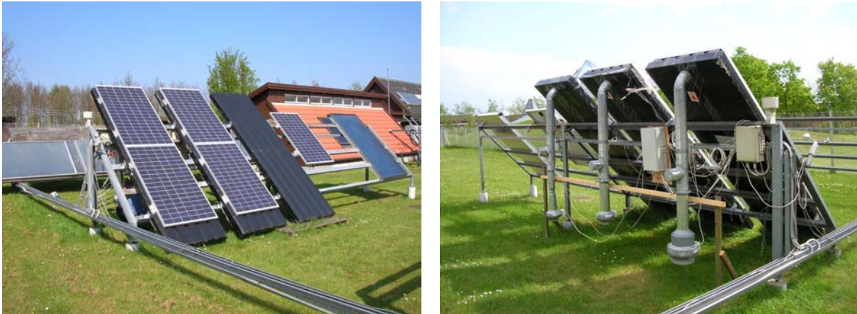
Figure 2. Front and back view of two SolarWall® PV/T transpired air collectors, one thermal reference and one PV reference in the test stand at the Danish Technological Institute .
