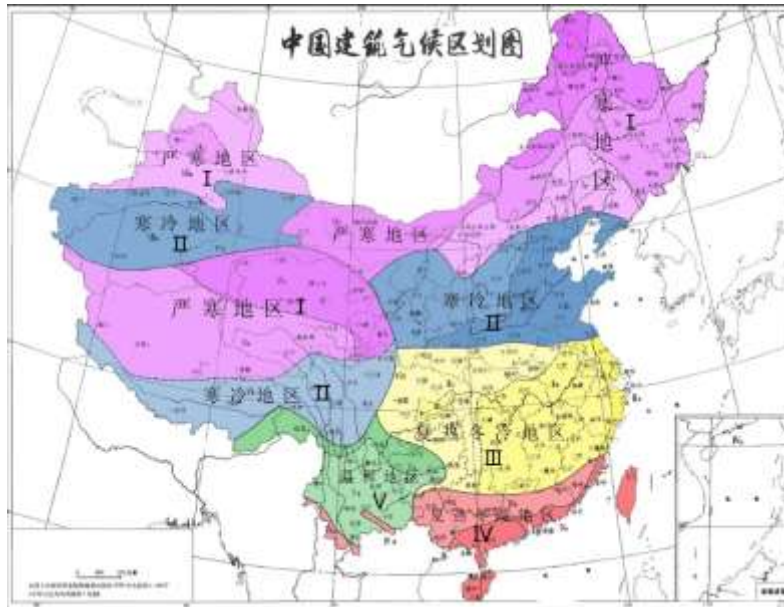
Figure 35. China Building Climate Zoning Map. Source: GB 50176-2016, Code for thermal design of civil building
