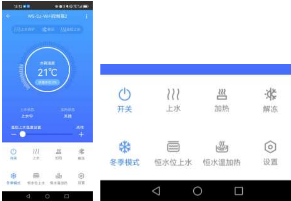
Figure 4: The Mobile Phone Control Interface of The Rooftop Solar Water Heater Controller (From Ma Guangbai (QIT)).
