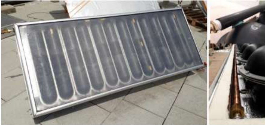
Figure 19: Left: Detailed Construction of The Single Loop System. Right: Full-scale Functional Model Out of Plastic Absorber-Storage Pipes. (Source: SolPol-4/5, Final Report, Climate and Energy Fund, Austria 2019).
