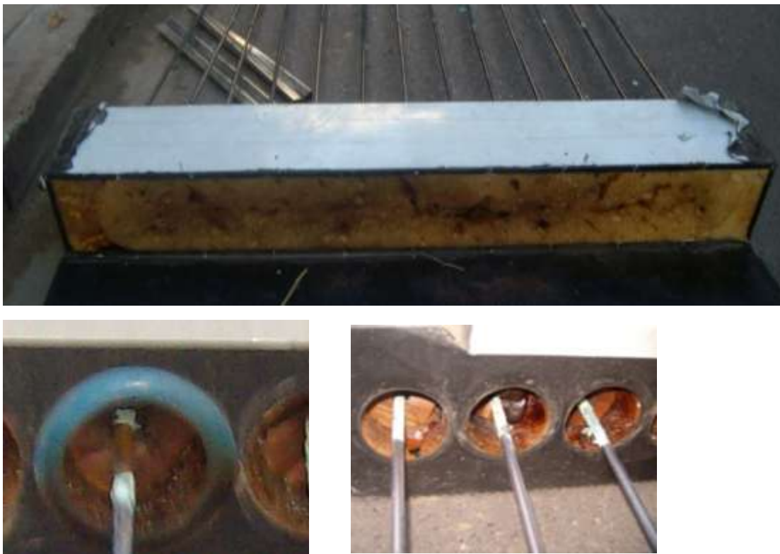
Figure 3: Images of Some ETCs after Exposure.
