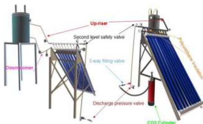
Figure 21: Front and Rear View of Solar Water Heating System with CO 2 Filling Circuit.
