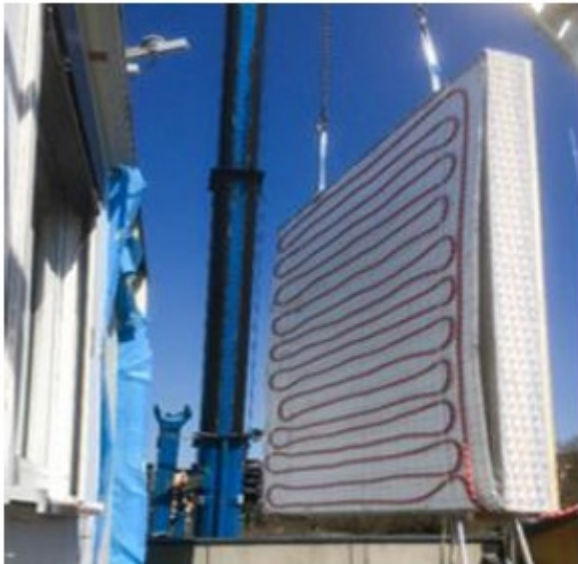
Figure 21: Velcro mounted heat dissipation system for building mass activation retrofit (left) and mounting of the prototype on the facade energy test rig at the laboratory of AEE INTEC (right), source AEE INTEC.
