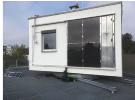
Figure 22: Active PV and heat dissipation layers of a multifunctional façade from EXCESS-Project (left) and the mounted prototype on the facade energy test rig at the laboratory of AEE INTEC (right), source AEE INTEC
